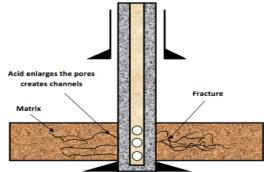
efficient inhibitors of acid corrosion up until the early 1930s, steel tubing in wells was shielded. As these inhibitors advanced through time, gas wells started to be treated with oil and acid more often. Today, one of the most popular and efficient technologies accessible to oil and gas operators for stimulating the productivity of wells is acidizing. Both new and aged wells undergo acidizing. It is carried out in old wells to enhance energy recovery and boost productivity.
