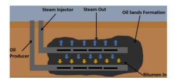
**SAGD in China.** The majority of China's super-heavy oil reservoirs are continental deposits with deep burial depths and significant heterogeneity, both of which significantly favor the use of SAGD technology. The first SAGD pilot test was conducted in the Guantao Formation and Hexing VI Formation in the Du84 block of the Liaohe oil field in 1996, followed by the drilling of the first pair of horizontal wells in the Shu1 region of
