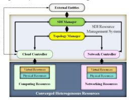
Fig. 2. High-level architecture of SDI RMS([7])
