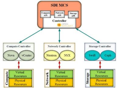
Fig. 4. SDI MCS connection to the laaS resource controllers
